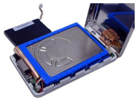
Set the hard drive back into the case and reattach the cable onto the logic board firmly. It may make a "click" as it's seated onto the logic board, that is normal, don't worry. You may find the attachment is performed more easily with the unit on it's side as you had it with the drive removal. Once complete, set the back cover onto the unit, being careful to make sure that the hold switch seats back over the internal switch properly.
