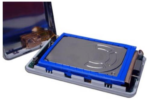
Once you have the bottom cover off, GENTLY tip it towards the top as shown. Be exceedingly careful of the ribbon connector that goes to the audio jack. It is easily damaged.
