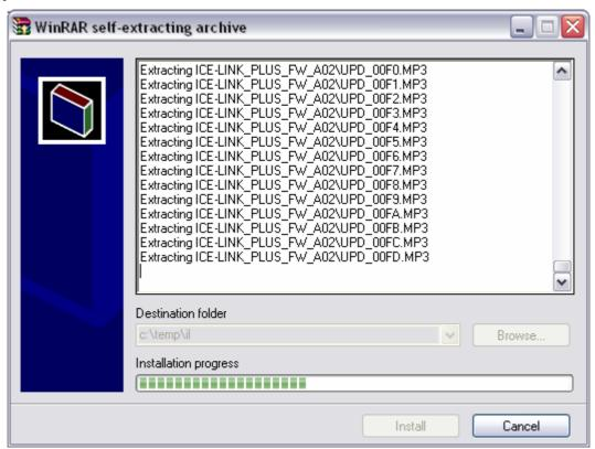
**a.** Copy the "ice-Link\_Plus\_fw\_xxx.exe" self extracting archive into a folder. Start the extraction by double clicking the file. A window, as shown in the image above, will open, showing the extraction process. For Mac ZIP format is also available.
